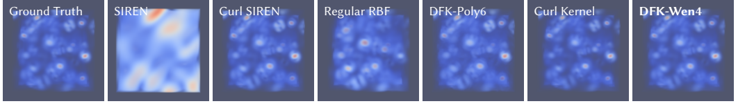
Fig. 2. Fitting experiments of the analytic vortices, with the resulting vorticity fields rendered. Physics-embedded methods clearly demonstrate superior fitting capabilities over physics-informed ones. Additionally, kernel-based approaches excel at capturing local details compared to neural network-based representations. Among all tested approaches, DFK-Wen4 achieves the lowest fitting error, as shown in Tab. 1.
